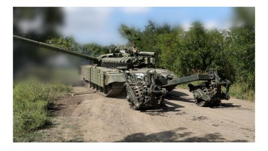
One set of rollers is 6.5 tonnes in weight and  $3.77 \times 3.44$  metres in size, and costs UAH2.5 million, including additional installation equipment. In total, the Group has already provided the army with dozens of its mine trawls. As for the additional equipment, it helps to significantly extend the service life of the rollers. In many cases, even damaged trawls at the front are suitable for prompt repair, so Metinvest produces and supplies spare components for them to Ukraine's military.
